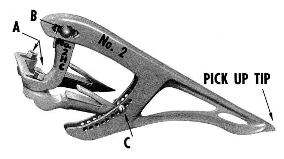
RAISE CUTTERBAR TO CONVENIENT WORKING POSITION AND ATTACH ONLY ONE CROP LIFTER AS DESCRIBED IN A, B, C, AND SPECIAL CUTTERBAR SETTINGS.
